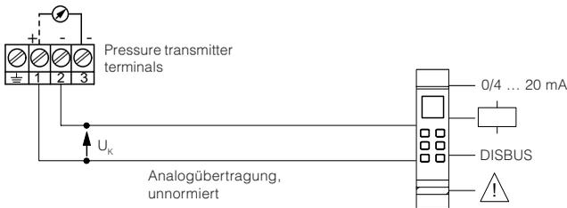
**Supply through a PLC with active input circuit**
