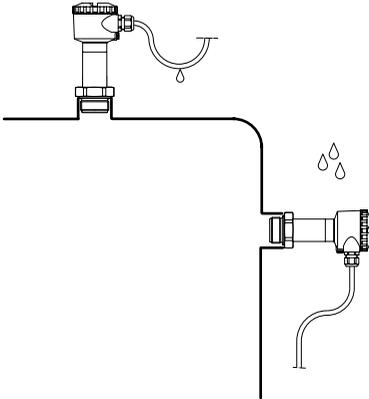
An appropriate connection seal must be used for mounting. This seal is either supplied with the pressure transmitter or must be provided by the customer.
