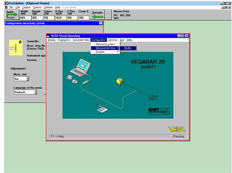
In the menu "Modify meas. loop configuration" you can give a name (e.g. vessel 10) and a description (e.g. cleaning detergent) to the measurement loop in place of the sensor number. This will make your entire measuring system more understandable.
