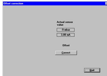
The example shows an absolute pressure transmitter with a measuring range of 0 ... 1000 mbar, with which low pressures (partial vacuum) are measured. The min. value was set to 50 mbar and the max. value (span) to 1000 mbar (i.e. the final value of the measuring range).
