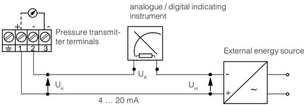
**Supply through a VEGA signal conditioning instrument**
