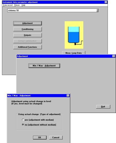
You can carry out the min./max. adjustment with or without medium. Generally you will carry out the adjustment without medium.
