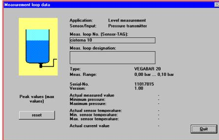
All available sensor information is displayed. With the button "reset" you can delete the pressure and temperature history saved in the sensor.
