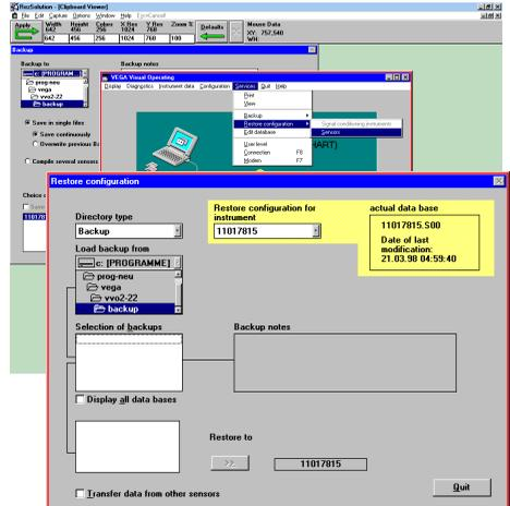
In this menu window, the actual setting (data base) with date and time of the last system configuration is displayed in the yellow window field. If you click on the serial number of the sensor from which you want to adopt the adjustments (in the yellow field), these sensor settings will be transferred to the currently connected sensor with "Restore to".
