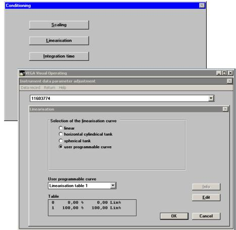
You can choose four linearisation curves: linear, horiz. cylindrical tank, spherical tank and user programmable curve.
