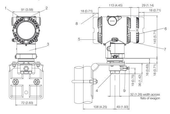
1 Adjustments | 2 Identification plate | 3 Certification plate | 4 Process connection | 5 Terminal side |6 Integral display housing | 7 Electronic side | 8 Space for cover removal | 9 Drain/vent valve
