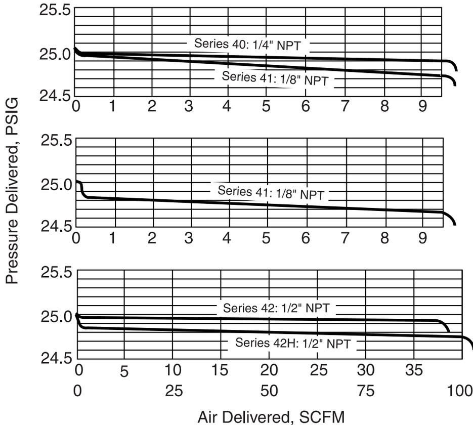
**Test Procedure:** Each 30-psig-range regulator was adjusted to 25 psig with 100 psig supply and no flow. Flow was increased to maximum capacity. All regulated pressure readings were taken at gauge connection in the body of the regulator.
